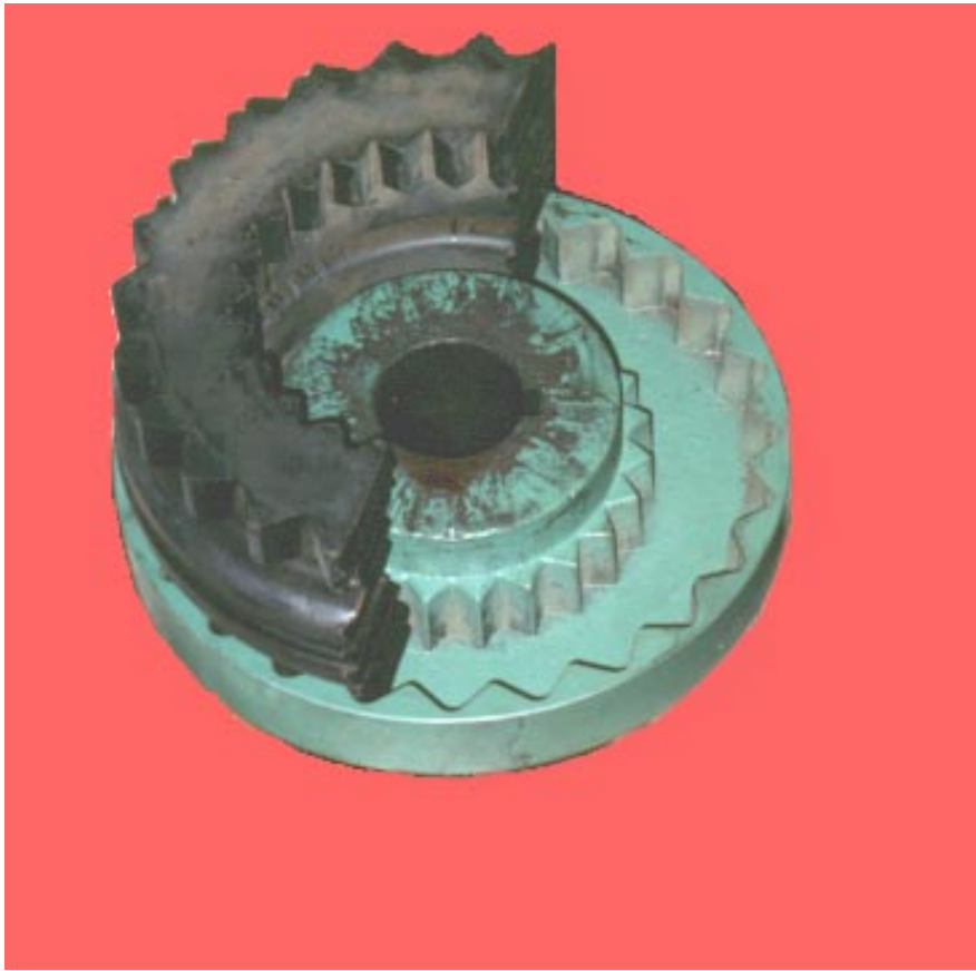
Figure 10. Motor coupling disassembled view.
