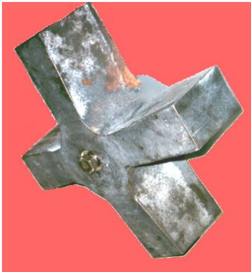
Figure 12. Rotor locking device installed for additional security.
