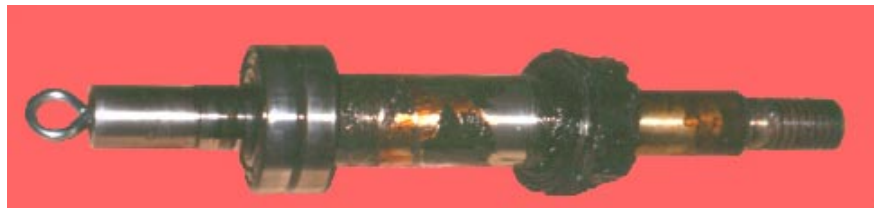
Figure 13. Replacement shaft/bearing assembly.
