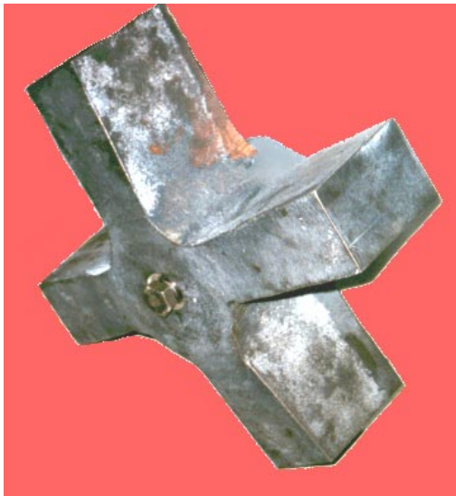
Figure 12. Rotor locking device installed for additional security.
